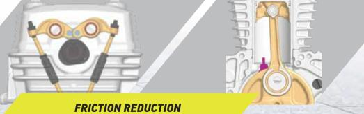
The piston cooling jet reduces friction and maintains optimum engine temperature. The offset cylinder and rocker roller arm further reduces the frictional losses in the engine.
